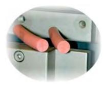
After breakage the load cell transfers to computer software the data which is then analysed and expressed in graph form and as industry standard MPa tensile strength.
